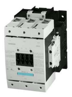
CONTACTOR, 55KW/400V/AC-3 AC(40...60HZ)/DC OPERATION UC 220...240V AUXIL. CONTACTS 2NO+2NC 3-POLE, SIZE S6 WITH BOX TERMINALS CONVENTIONAL OPERATING MECHAN. SCREW TERMINAL
