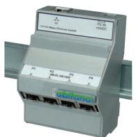
The 5 port 10/100Mbps Switch automatically recognises all attached network equipment and chooses the highest possible bit rate (10 or 100Mbps) and transmission mode for each equipment. The auto MDI/MDIX function eliminates the need (and risk of errors) for crossover patch cords. This unit requires 5VDC from a power supply ABI-PS1001S14.
