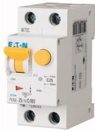
**FI/LS, 16A, 30mA, miniature circuit-breaker trip curve C, 1pole+N, residual current circuit-breaker trip characteristic: A**
