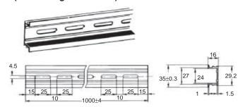
\* A total of twelve  $25 \times 4.5$  elliptic holes is provided with six holes cut from each track end at a pitch of 10 mm.
