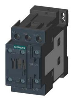
CONTACTOR, AC-3, 15KW/400V, 1NO+1NC, DC 24V, 3-POLE, SZ S0 SCREW TERMINAL
