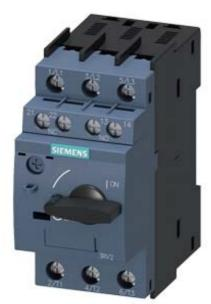
DISJONCTEUR TAILLE S00, POUR PROTECT. MOTEUR, CLASS 10, DECL.A 1,8...2,5A, DECL.N 33A BORNES A VIS, POUVOIR DE COUPURE STANDARD, BLOC CONT. AUX. TRANSV. 1NO+1NF
