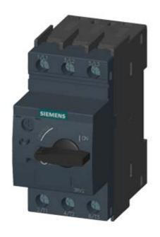
CIRCUIT-BREAKER SZ S0, FOR MOTOR PROTECTION, CLASS 10, A-RELEASE 17...22A, N-RELEASE 286A, SCREW CONNECTION, STANDARD SW. CAPACITY,
