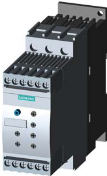
SIRIUS SOFT STARTER, S0, 12.5A, 5.5KW/400V, 40 DEGR., AC 200-480V, AC/DC 24V, SCREW TERMINALS
