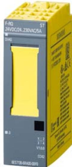
SIMATIC DP, MODULE ELECTRONIQ. POUR ET200SP, F-RQ 1X 24VCC/24..230VCA/5A ST, 20MM LARGEUR, 1 SORTIE RELAIS (2 NO) COURANT SORTIE TOTAL 5A, TENSION CHARGE DC 24V ET CA 24 .. 230V, PEU ATTEINDRE PL E (ISO 13849-1: 2008)/ SIL 3 (IEC61508: 2010) SI COMMANDE PAR F-DQ (P.E. 6ES7136-6DB00-0CA0)
