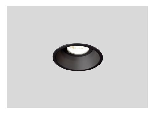
Round ceiling recessed downlight made from die-cast aluminium; surface Jet Black; powder coated; matt texture; RAL 9005; installation without tools using wire springs; suitable for ceiling thickness of 4-25 mm;  $recessed\ depth\ 105\ mm; lamp\ socket\ GU10; lamp\ type\ PAR16; max.\ 12W; 100-240\ V; degree\ of\ protection$ IP44; PC2; UGR 16; VDU compatible workplace luminaire according to DIN EN 12464-1; luminance above  $65^{\circ}$  1500 cd/m<sup>2</sup>; lamp not included;
