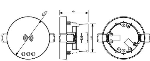
821006001800 - LEDSmart-BLE2-Rc-MW-Sensor
